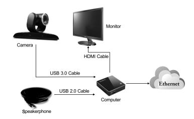
▼ Video Conference - connecting to dual monitor Camera System Switch should be set to USB Mode
